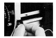
When installing the distance scale, insert the shaft end opposite the revolving knob into the camera body bearing. Insert the shaft end while pressing the spring located near the bearing to the inner side with the side of the scale. Next, fit the shaft to the front bearing while pushing in the shaft tip with a finger nail; then install the cover as it originally was.
